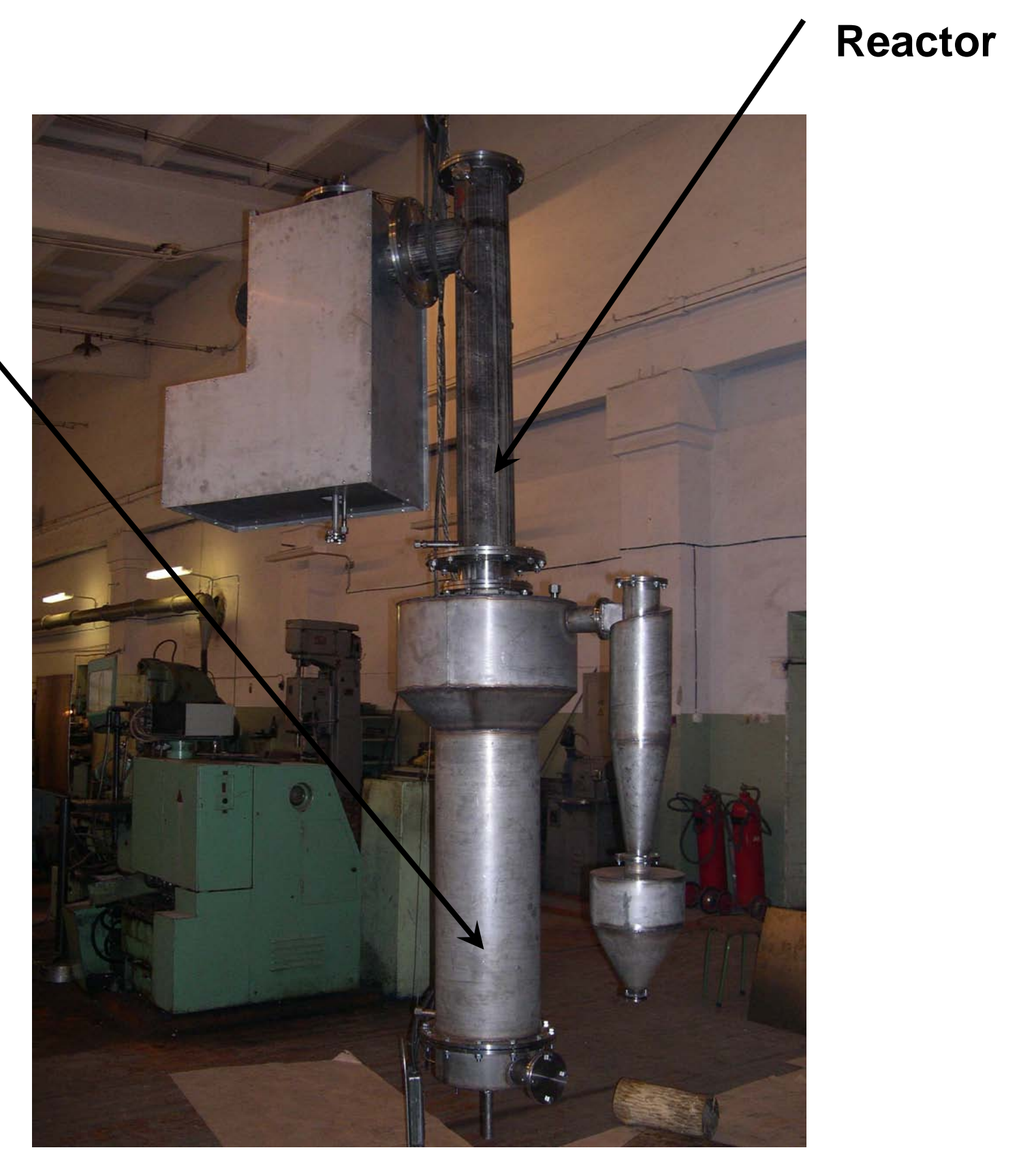
Pilot plant for testing the catalysts under realistic conditions
